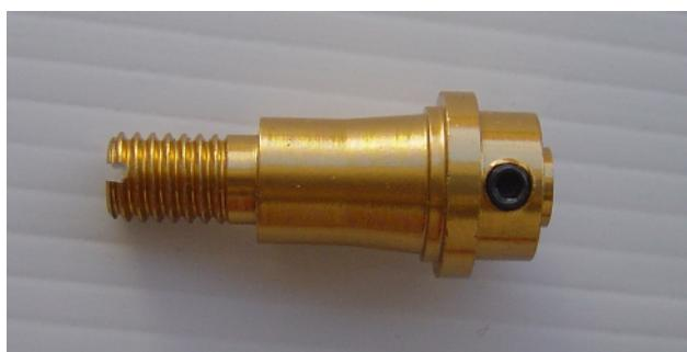
Cut a slit into the fan rotor adapter on the end with the thread. It's easy to do this with a hacksaw.
