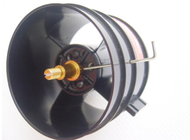
Press the fan rotor adapter onto the motor and tighten the hex screws against the shaft. Be sure to place one of the screws at the position of the flattened motor shaft. Use a small amount of Loctite 222 or similar to secure the screws.
