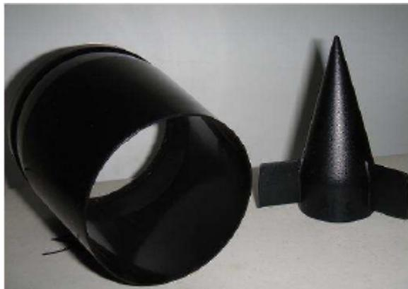
The WM 400 thrust nozzle and exit cone comes in two parts. The cone is assembled inside the thrust nozzle with epoxy glue.
