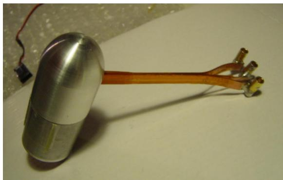
Another possibility to connect the motor wires is to use copper stripes. You may use this method with or without the use of the motor cone. Pay attention for a proper isolation between each copper stripe as well as between copper stripes and motor case and/or motor cone.
