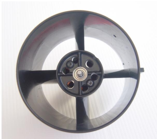
Slide the motor into the motor housing and fix the motor with two screws. Use a small amount of Loctite 222 or similar to secure the screws.
