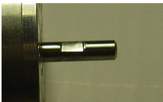
To avoid spinning of the Motor shaft, flat on the motor shaft.
