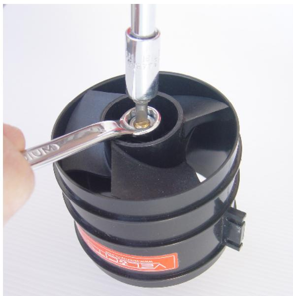
Fit the rotor over the fan rotor adapter. Slide the washer from aluminium over the adapter and tighten the hex nut as shown on the picture. Use a small amount of Loctite 222 or similar to secure the hex nut.
